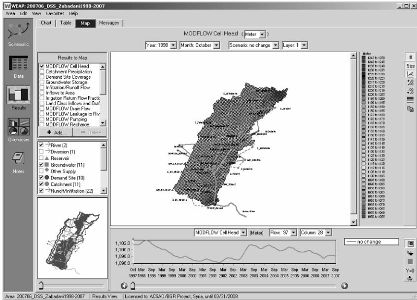
Fig. 3.1.13. Calculated hydraulic heads in the scenario 1998-2007.
