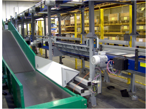
Fig. 8. Discharge element; unloads a tote by tilting it, so the bag falls onto a conventional conveyor belt
