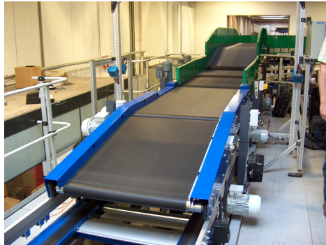
Fig. 4. Toploader element; an empty tote is ready underneath the traditional conveyor belt, where the bags will arrive
