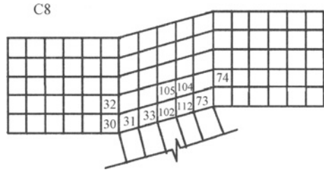
Figure 4. C8 failure place & sequence
