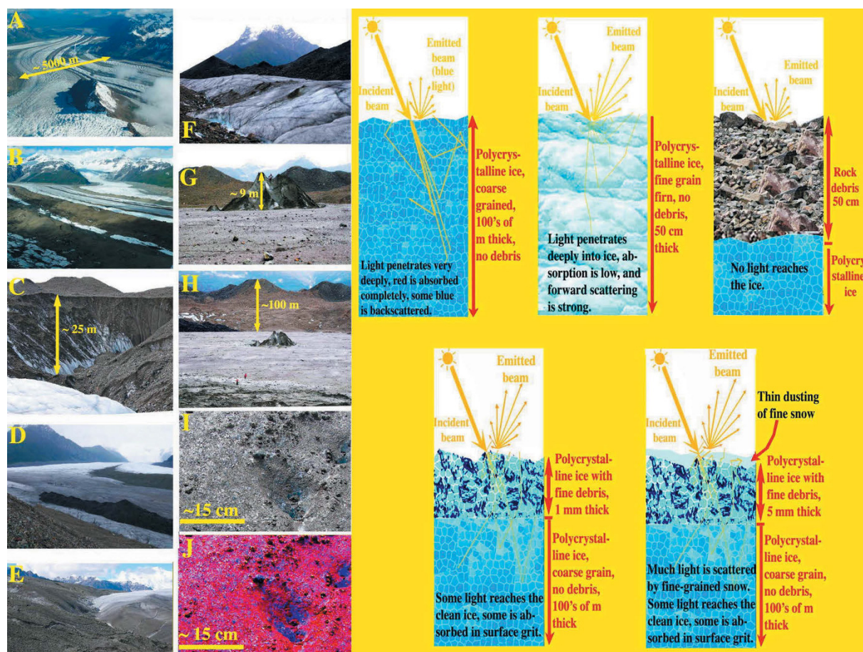
Figure 3.1. (A–J) Examples of monomineralic and monolithologic materials, intimate mixtures, and areal mixtures of materials on the Root and Kennicott Glaciers in the Wrangell Mountains, Alaska. On the right side of the figure are illustrated a set of typical scenarios that can be modeled using multi-layer 1D, two-angle radiative transfer equations (eq. 3.3). The geometrical configurations include single-layer and multi-layer arrangements of mixtures of ice and rock debris. Figure can also be viewed as Online Supplement 3.1.
