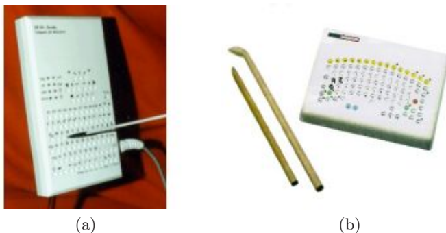
Fig. 2. Specific keyboards for handicapped people using a stem with mouth: M32h keyboard by SEVEKE (a) and GT keyboard by GORLO (b)
