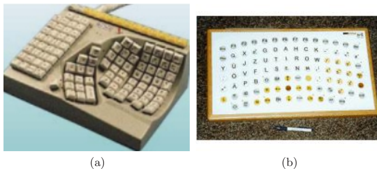
Fig. 3. Other examples of adapted keyboards: ergonomic keyboard MALTRON for right hand (A) and improved keyboard SUMO (b)
