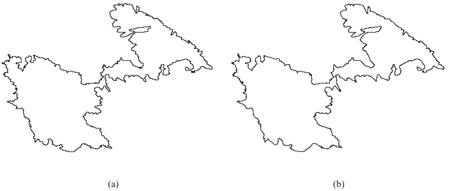
Fig. 14. (a) Coastline E (Astypalaia) consisting of 7510 points. (b) The reconstructed curve using FCF method with r = 1:6.68 .
