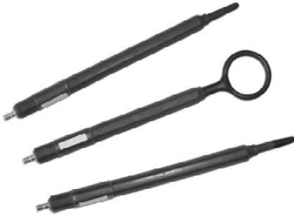
Fig. 3. Near-field probes that have been used for the measurements
