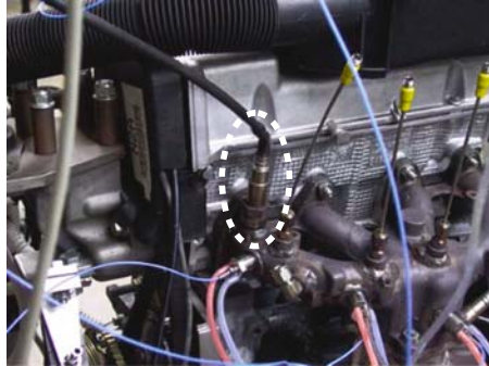
Fig. 7. Location of the UEGO sensor (dotted oval)
