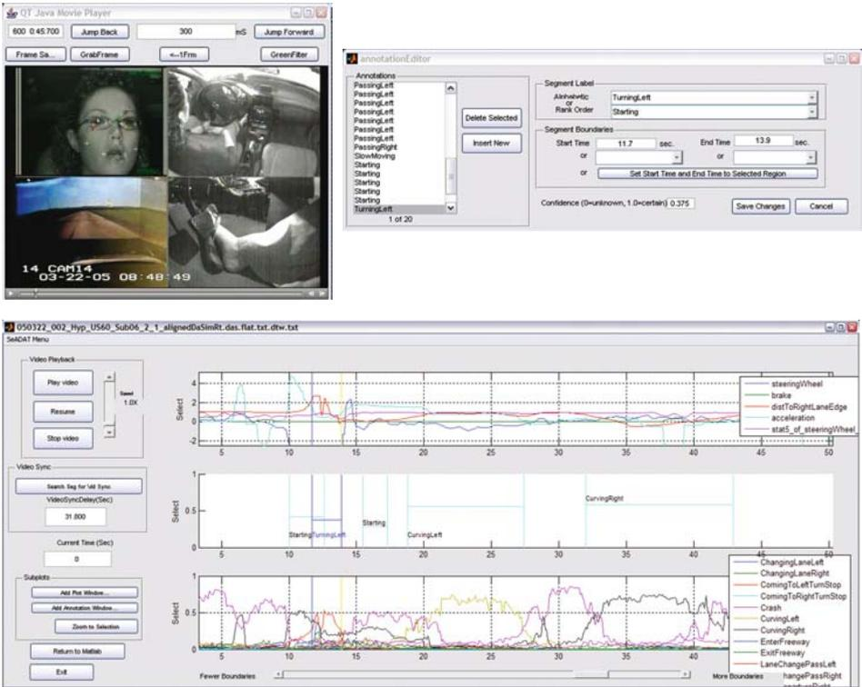
Fig. 2. The annotation tool. *Top left*: the video playback window. *Top right*: annotation label window. *Bottom*: sensor signal and classifier result display window. Note that colors have been re-used. See Fig. 5 for a complete legend
