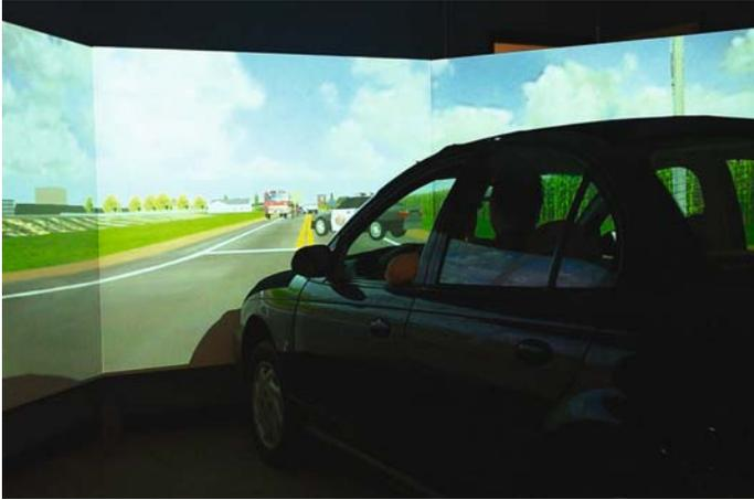
**Fig. 1.** The driving simulator
