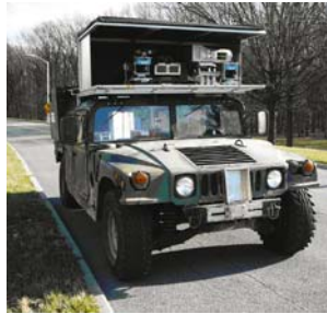
Fig. 3. ARL/NIST HMMWV Testbed showing several sensors mounted above the cab
