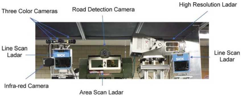
Fig. 4. Sensor suite mounted on the HMMWV cab
