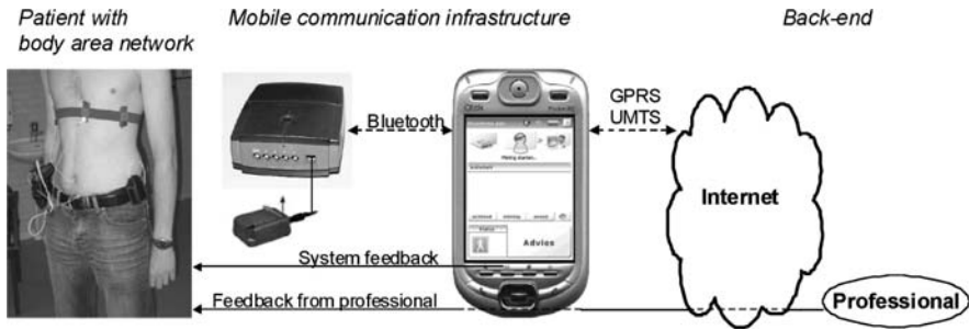
Fig 16.1. Schematic presentation of the service concept for chronic lower back pain patients (Van Weering et al., 2007)
