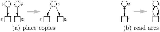
Fig. 3. Graphical conventions used to simplify patterns. (a) A dashed place is a copy of a place with the same label. (b) Read arcs are unfolded to loops.
