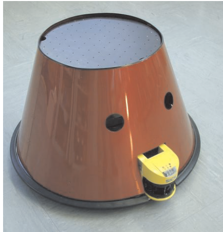
Fig. 2 The prototype of AGV used in the experiment.
