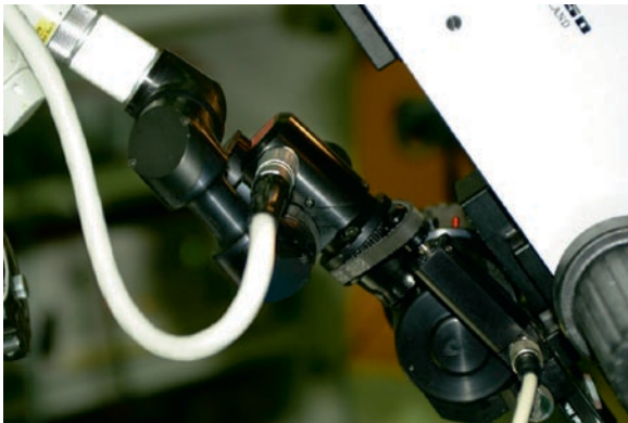
Fig. 4b.1. Scanning device connected to the laser arm and the micromanipulator. The scanning device is guided by the Acublade software
