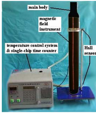
Fig. 2 MF magnetoviscous effect experimental instrument
