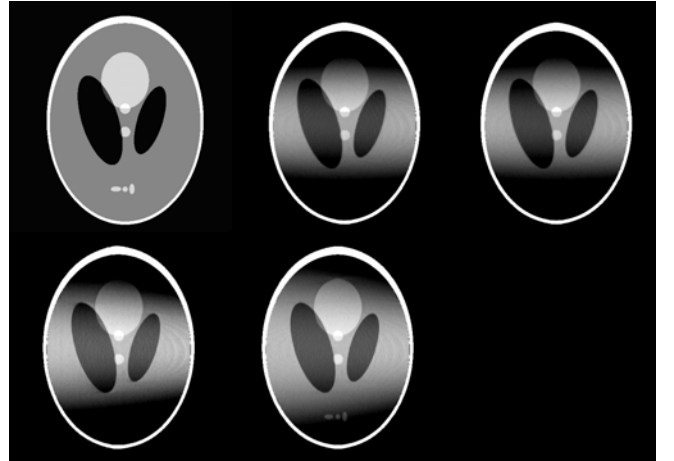
Fig. 3 Sagittal slices in 3D images, reconstructed images using the FDK algorithm( first row middle),the weighting function FDK(first row right) reconstructed images using the FDK half scan (second row left ), the weighting function proposed in this paper (right). (Window Width=15,Window Level=88)
