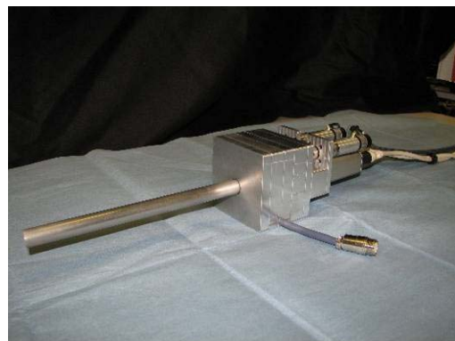
Fig 1 Wedge prism 3D endoscope
