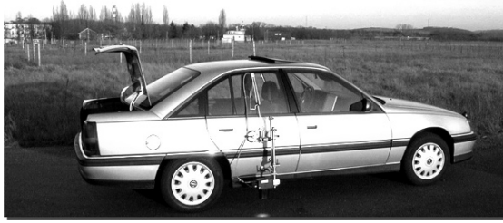
Fig. 24.63. Car for driving experimental for model validation and parameter estimation
