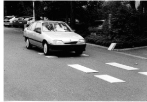
Fig. 24.64. Driving experiment with wooden plates to excite the vertical dynamics
