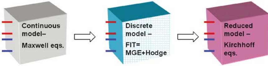
Fig. 1. Three levels of abstraction for a component model and its corresponding equations.
