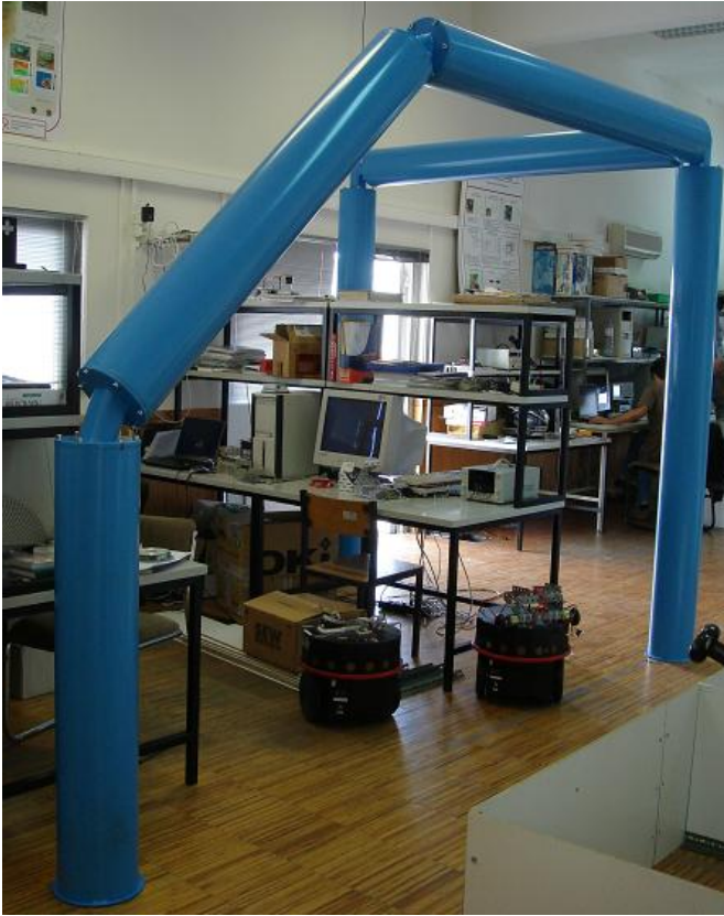
Fig. 3. Developed structure for Pole Climbing Robot Benchmarking
