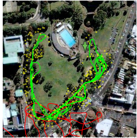
Fig. 6. The built map on the Victoria Park dataset by using the IFRM algorithm. The red line is the raw odometry trajectory. The green line is the estimated robot trajectory. The yellow stars are the estimated locations of observed objects (e.g. trees, human)
