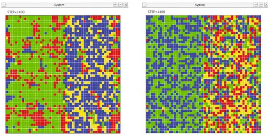
Fig. 10. Snapshot of agent configurations at 1400 time steps when simulation is carried out with the parameters listed in Table 7, except for failure rate and repair rate \mu = 0.5 , where strategic repair ( left ) and uniform repair ( right ) are compared
