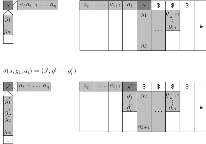
Fig. 6.29. A non- \lambda -transition of the pushdown automaton \mathcal{M} (left) and the corresponding transition of the OCA \mathcal{M}' (right). Counters are not depicted.
