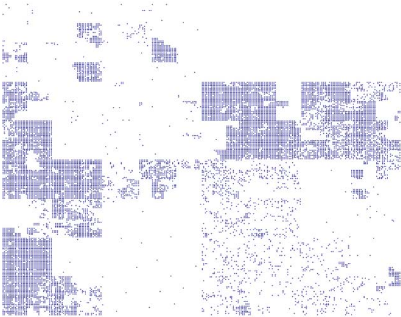
Fig. 5 Plot of eighth order representation of the data in Fig. 4, showing buckets corresponding to /16 networks (Class B)
