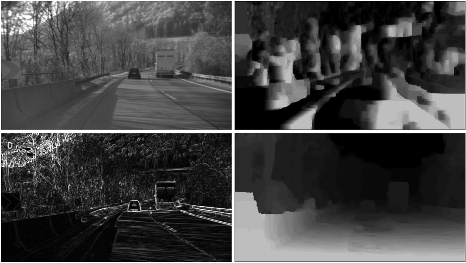
Fig. 6. Image 0227_c0 of Sequence 4 (upper left) and its associated BP result (upper right). The Sobel edge image (lower left) and the corresponding BP result (lower right).
