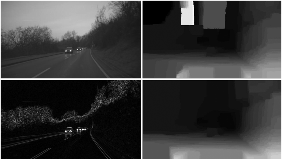
Fig. 5. Image 0001_c0 of Sequence 3 (upper left) and its associated BP result (upper right). The Sobel edge image (lower left) and the corresponding BP result (lower right).
