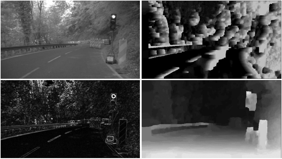
Fig. 8. Image 0001_c0 of Sequence 6 (upper left) and its associated BP result (upper right). The Sobel edge image (lower left) and the corresponding BP result (lower right).
