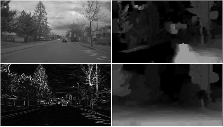
Fig. 4. Image 0001_c0 of Sequence 2 (upper left) and its associated BP result (upper right). The Sobel edge image (lower left) and the corresponding BP result (lower right).
