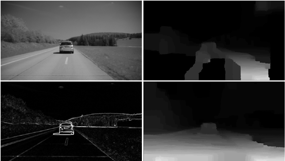
Fig. 7. Image 0001_c0 of Sequence 5 (upper left) and its associated BP result (upper right). The Sobel edge image (lower left) and the corresponding BP result (lower right).
