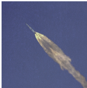
Fig. 1. Diverging exhaust plume of the Saturn V Launcher
