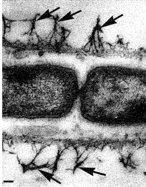
Fig. 6. Thin section of Leptothrix sp. which is precipitating manganese oxide on its outermost structure called a sheath (McLean et al. 2002). The arrows point to the manganese mineral phase identified by EDS. Scale bar = 150 nm.
