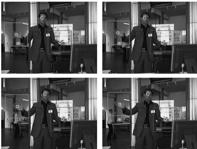
Fig. 15.2. In this tracking sequence head and hands were found. The identity of the objects is visualized by the gray value of the rectangles, which delineate the search region of each tracking agent. Moving skin color in the background is ignored.
