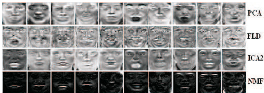
Fig. 14.3. Holistic subspace image representation. From top to bottom, each row depicts the first 10 basis images (out of 49) corresponding to PCA, FLD, ICA2 and NMF. For PCA the basis images are ordered by decreasing variance, for ICA2 and NMF by decreasing kurtosis.
