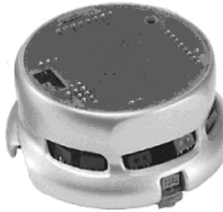
Fig. 10. The miniature mobile robot: Khepera
