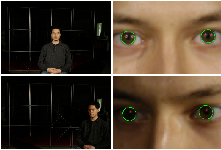
Fig. 5. A subject at different locations and orientations relative to the camera and two light sources. Shown to the right are magnified views of the eyes. The ellipse fit to each limbus is shown in dashed green and the red dots denote the positions of the specular highlights. See also Table 1
