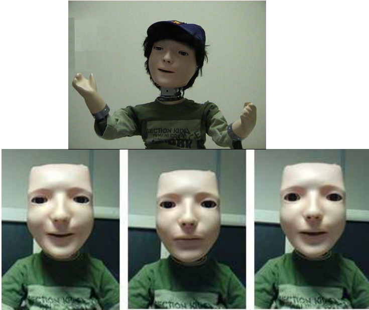
Fig. 3. The child-sized humanoid robot KASPAR [51] used in the European IST-FP6 Robot-Cub project [52] investigating human-robot interaction, specifically issues regarding interaction kinesics, imitation, and computational architectures for a robot to extend its temporal horizon via interaction histories [45]. The aim of designing KASPAR was to study what types of human-robot interactions a minimal set of expressive robot features can afford 4 . The goal is not perfect realism, but sufficient realism for rich interaction. KASPAR has 8 degrees of freedom in the head and neck and 6 in the arms and hands. The face is a silicon-rubber mask, which is supported on an aluminum frame. It has eyelids and 2 DOF eyes fitted with video cameras, and a mouth capable of opening and smiling.
