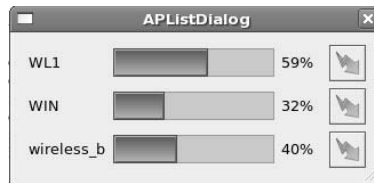
Fig. 5. This graphic interface will display wireless signal strength of APs that a mobile device can attach. For example, this figure displays three signal strengths of AP including WL1, WIN and wireless_b.
