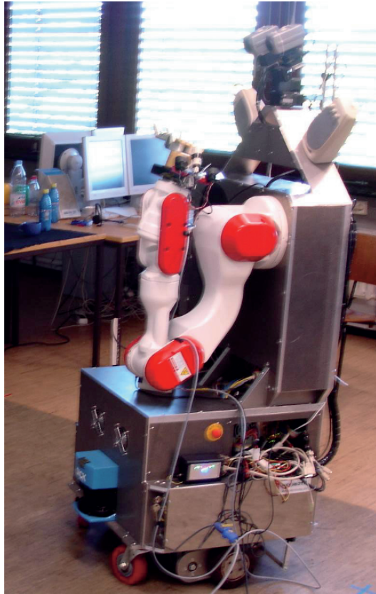
Fig. 10.16. The mobile robot setup in our laboratory for dexterous manipulation
