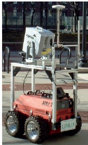
Fig. 3.4. The ATRV-2 based AVENUE mobile robot for automated site modeling (Blaer and Allen 2006)
