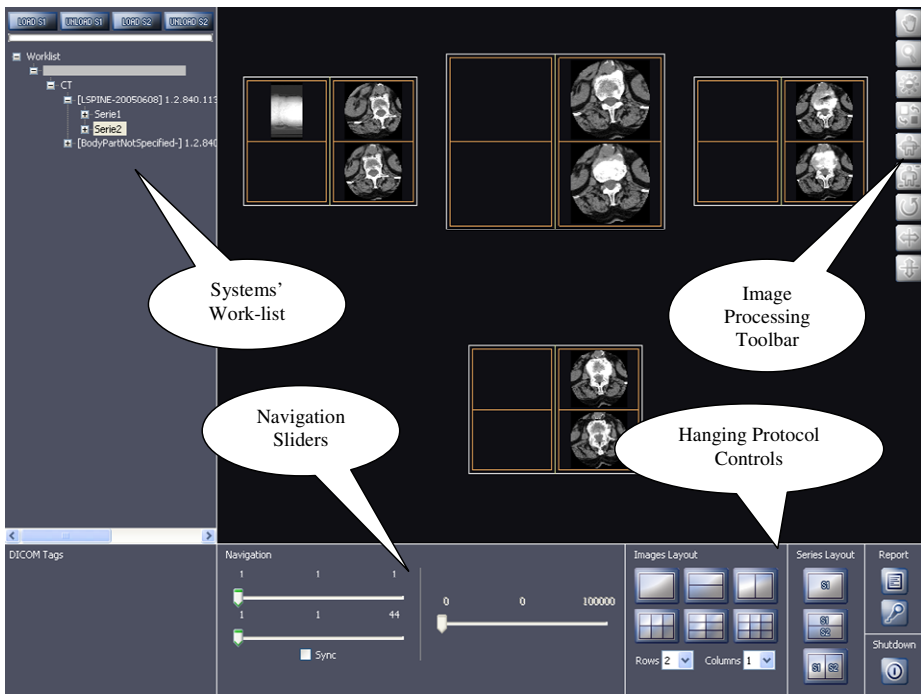
Fig. 4. Control Station Interface where the Systems' Work-list (presenting only one blanked patient with two CT studies), Navigation Sliders, Image Processing Toolbar and the Hanging Protocol Controls are pointed out
