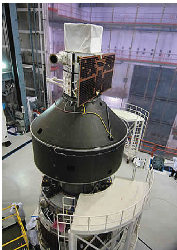
Fig. 23.12 The AGILE satellite integrated on the fourth stage of the PSLV rocket (15 April 2007). Launch on 23 April was successful, and an image of the Vela pulsar was made public on 29 May (Image courtesy of ASI)
