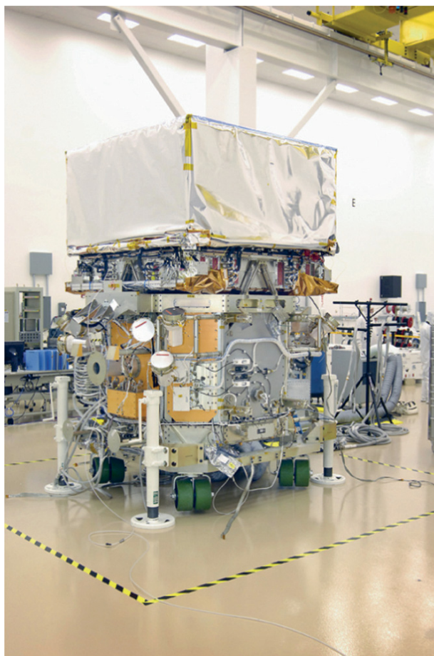
Fig. 23.3 The Large Area Telescope mounted on the (then incomplete) GLAST satellite, December 2006 (Image courtesy of NASA/General Dynamics)
