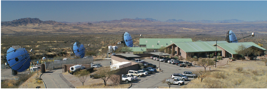
Fig. 23.2 The four telescopes of the VERITAS Cherenkov imager array in January 2007 (Image courtesy of VERITAS Collaboration)
