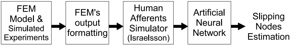
Fig. 1. Block diagram of the software modules
