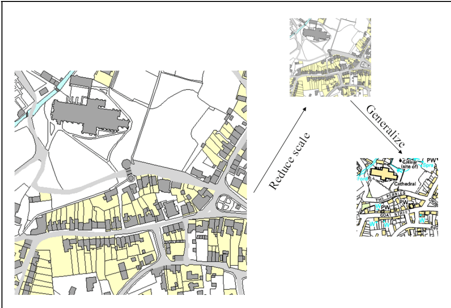
Fig. 1. Example of generalisation brought about by a change in scale. Data sets shown are OS Mastermap (large scale) and OS 1:50,000 raster for the St. David's area, West Wales.
