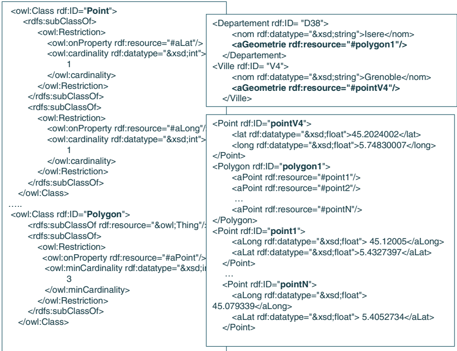
Fig. 1. The geometric description of a department and a city using the OWL language
