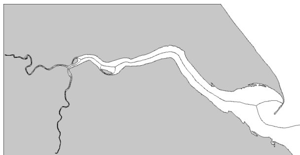
Fig. 2. The results of contour partitioning to reduce the medial axis of the Hull Estuary to a simplified skeleton whilst retaining topology of the shape
