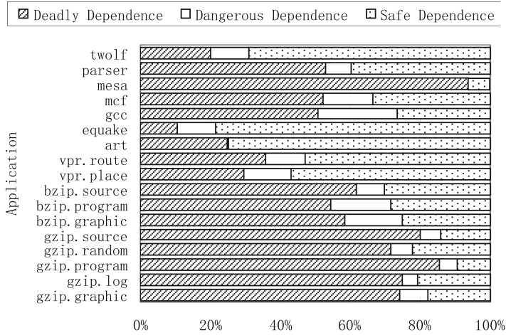
Fig. 8. Memory dependence distribution for loop speculation
