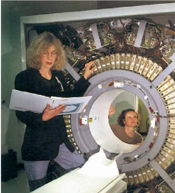
Fig. 6.6 The typical PET scanner with ring detector configuration
