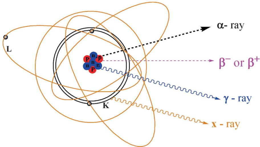
**Fig. 4.1** The three components of radioactive emissions originating from the unstable nuclei of natural radionuclides of uranium and thorium:  $\alpha$ ,  $\beta^-$  and  $\gamma$ , as they were called by Rutherford.
