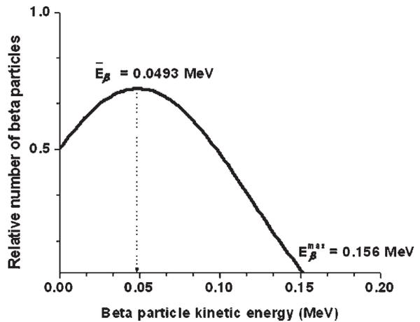
**Fig. 4.3** The continuous  $\beta^-$  energy spectrum showing the distribution of  $\beta^-$  particles (relative number versus energy) emitted by  ${}^{14}\text{C}$ . The average energy is denoted by  $\bar{E}_\beta$ , while the maximum energy is denoted by  $E_\beta^{\text{max}}$
