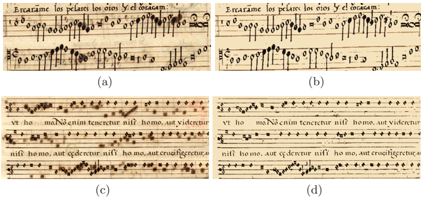
Fig. 2. Results of processing two of the original images with the proposed method. The first column presents the original images, while the second shows the restoration results.
