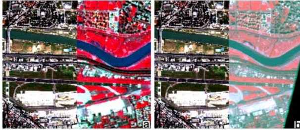
Fig. 8. Overlapping of the reference and registered working images in the “Multi-sensor” case. (a) The registration results of Image 1. (b) The registration results of Image 2.
