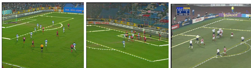
Fig. 2. Effects of non-linear refinement: grey lines are projected using the estimate of H computed by the linear method; white lines are projected using the refined estimate. The white circles are the inlier warped points \pi_{k,l}^* .
