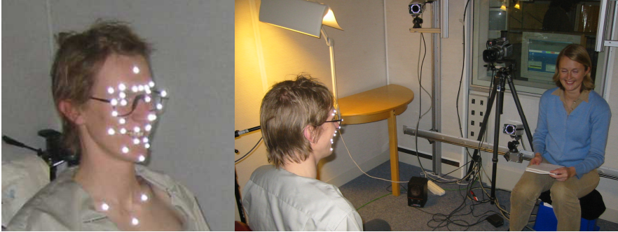
Fig. 3. Data collection setup with video and IR-cameras, microphone and a screen for prompts (right) and test subject with the IR-reflecting markers glued to the face (left)
