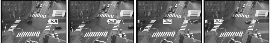
Fig. 5. MERL traffic video sequence ( x \times y \times t = 368 \times 240 \times 64 ) where a white car is tracked as it travels through an intersection. From left to right frames 13, 24, 38, and 58 are shown. Tracked regions are highlighted with white boxes.
