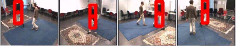
Fig. 2. The particle distributions in four cameras at a time instant. It can be seen that the foot positions are not precise although all the particles are placed at the right location.
