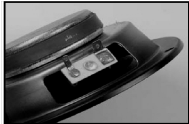
Fig. 14.2. The wire that runs through the speaker system connects to two hook-up jacks on the driver.
