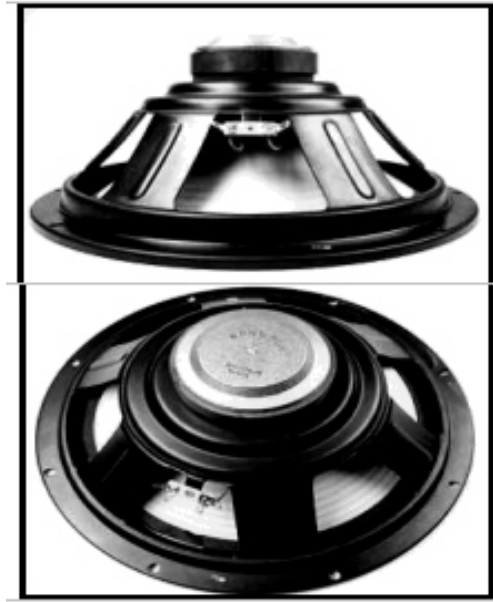
Fig. 14.1. A typical speaker driver, with a metal basket, heavy permanent magnet and paper diaphragm
