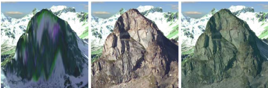
Fig. 4 The images show a screenshot of the textured elevation model ( left ), with a photo mapped on it ( middle ) and with applied histogram matching and blending ( right )
