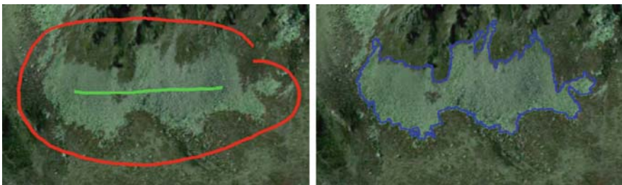
Fig. 7 Landform mapping based on a graph cut optimization. The left image shows the initial user input marking foreground and background regions. The right image shows the segmentation result automatically computed from the user input
