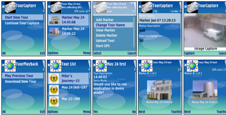
Fig. 6. Mobile phone tour prototype user interface. The tour capture interface is shown along the top row, and the tour playback along the bottom row.
