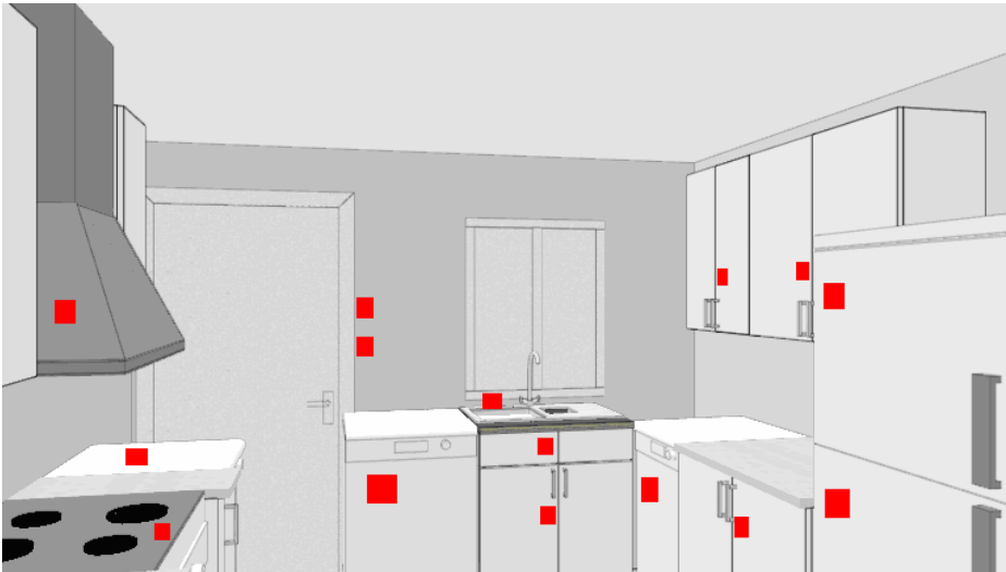
Fig. 6. Graphical representation of the kitchen where the experiments were carried out, showing the locations of some of the sensors
