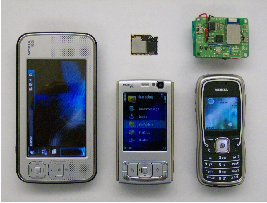
Fig. 4. Mobile devices currently integrated into the CenceMe system: the Nokia N800 Internet Tablet, Nokia N95, Nokia 5500 Sport, Moteiv Tmote Mini (above the N95), and prototype BlueCel accessory (above the 5500)
