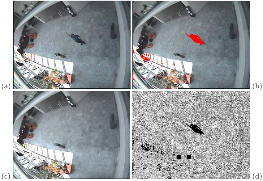
Fig. 3. Results of HSV-SO algorithm on Walk1 sequence: (a) original frame; (b) original frame with moving object detection mask; (c) background model; (d) background model change mask from previous frame
