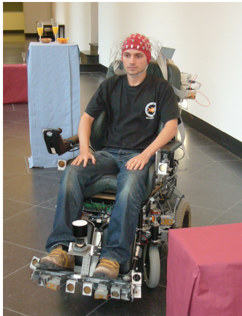
Fig. 3. Subject driving the wheelchair in a natural environment from non-invasive EEG. Note the laser scanner in front of the wheelchair, in between the subject's legs.
